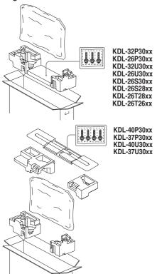
5 Fix the TV to the stand using the supplied screws.
